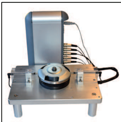
Capacitive probes connected to a D200S
