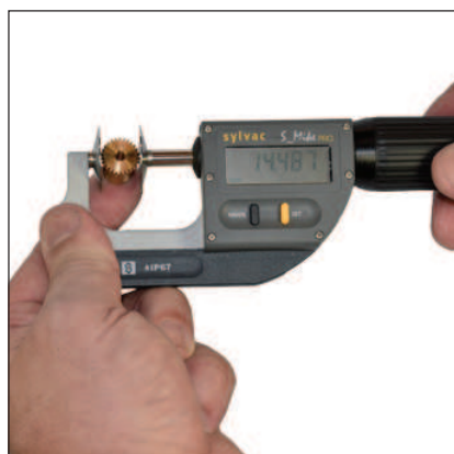
Part measurement with a S_Mike PRO Disk
