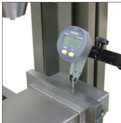
Checking the alignment on milling machine.
