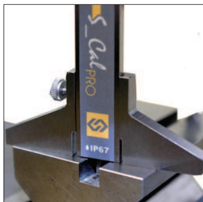
Depth measurement with S_Cal PRO and base 910.2205.
