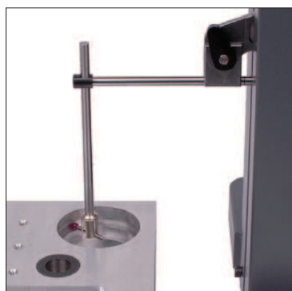
Internal groove measurement with accessories 930.2108, 930.2110 and 905.2207
